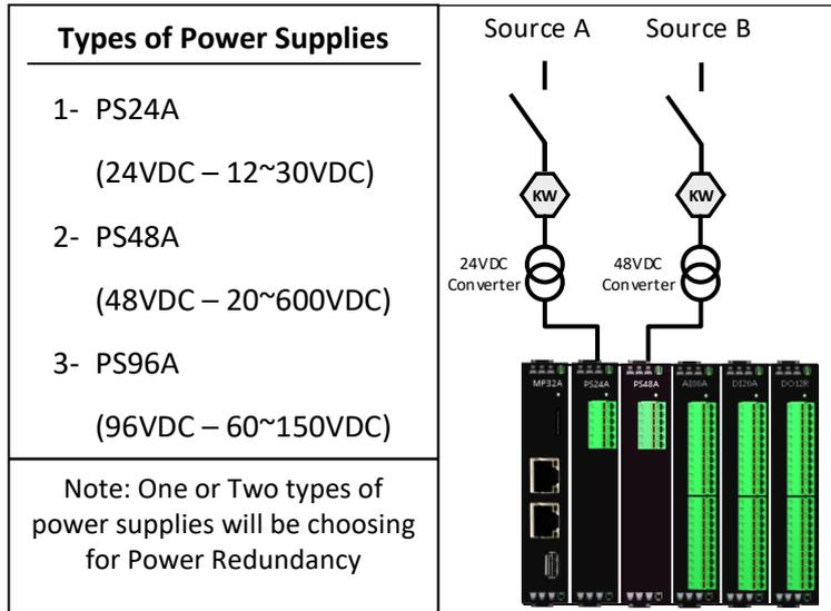
Note: The system can be sourced by two different power sources.
