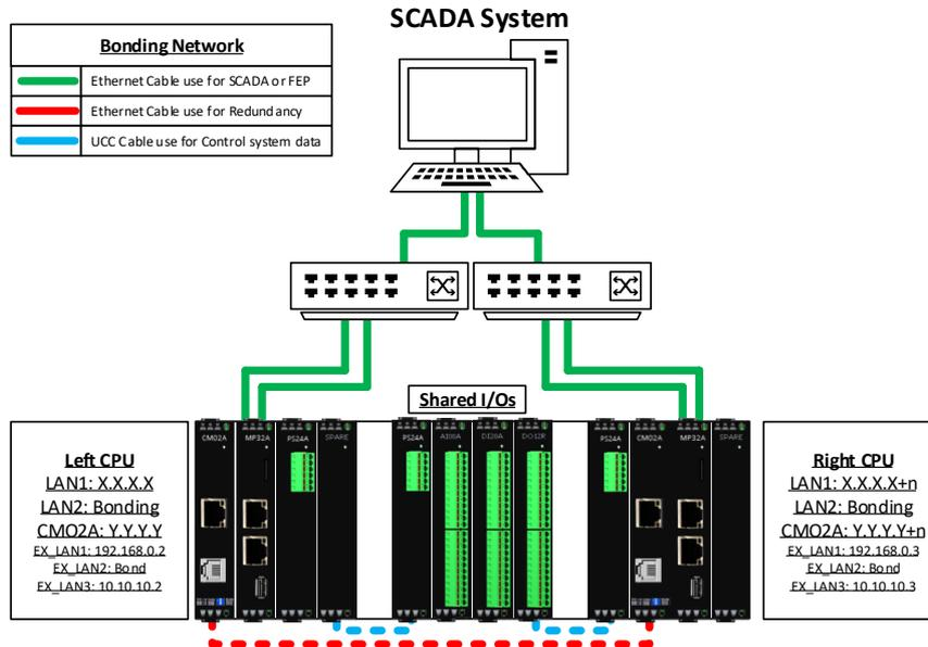
Setup IP addresses on both of RTUs and enable redundancy function on them.
