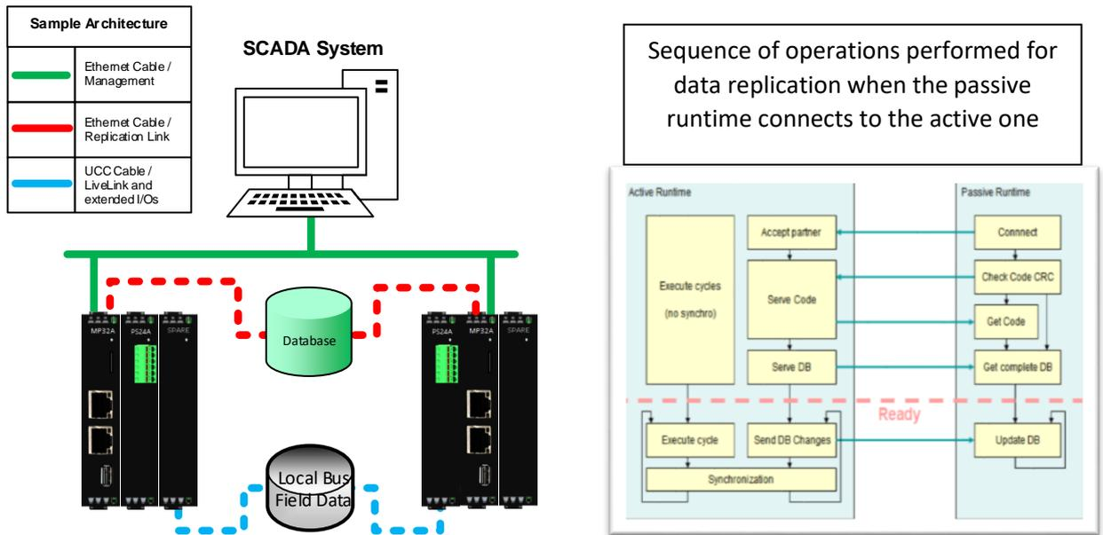
Management Link: Available connection to communicate with upstream systems, like SCADA or FEP
