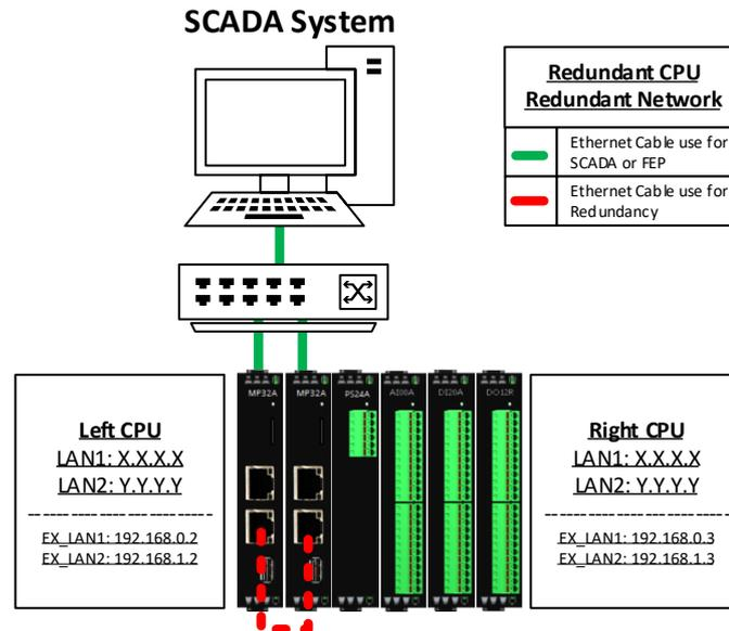
Setup IP addresses on both of RTUs and enable redundancy function on them.
